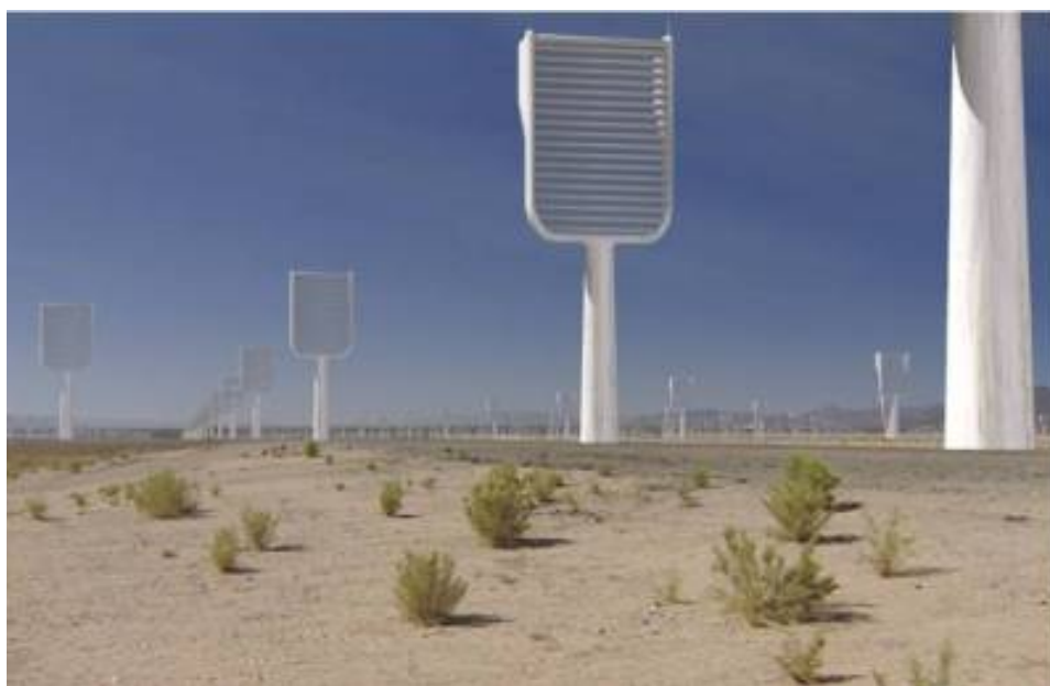
Fig. 5. Moisture swing absorption (single step) technology
